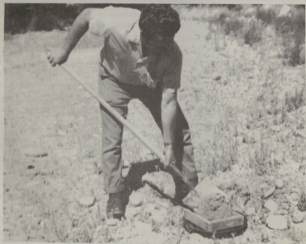
FIGURE 16: (1st minute) Shoveling gravel into screen.
