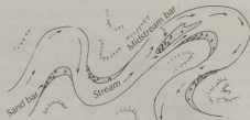
FIGURE 6: Gold is supposed to concentrate on the inside of river bends (A) and on upstream part of mid-stream bar (B). But when the entire valley contains gravel from glacial outwash, all of the gravel may have been on the inside of a bend at some time in the past.
