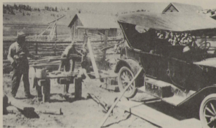
This device was used for wood sawing and cycle grinding. Author's collection.
