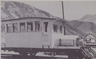
Casey Jones at Eureka, 1940. It originally had a Maxwell motor and was intended to serve as an ambulance. It soon appeared in other capacities, though, making the 20 minute run from Eureka to Silverton. Casey was eventually equipped with a Cadillac engine, could seat 11 passengers. ( Denver Public Library, Western History Department )
