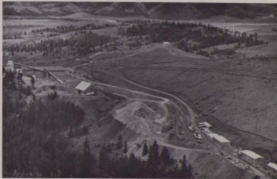
Aerial view of the Homestake Mining Company's new Bulldog mine and silver-lead concentrating mill at Creede. Construction of the 300-ton per day mill was completed in March of 1969. Homestake employs seventy persons in its Creede complex.
